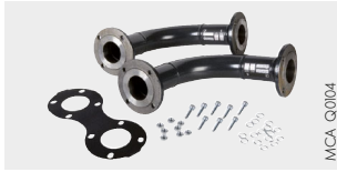
Set of DN 65 90° elbows for cascade systems from 304 to 455 kW - Package HC209 Set of DN 100 90° elbows for cascade systems from 460 to 608 kW - Package HC210 Supplied with gaskets, nuts and bolts. Enabling the low-loss header to be connected perpendicular to the manifold.
